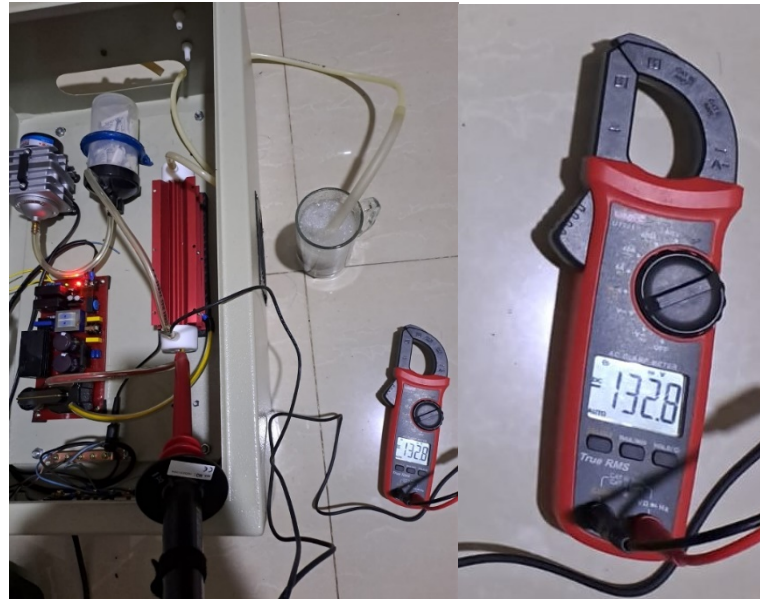
Figure 8. High voltage measurement with a frequency of 100 Hz.
