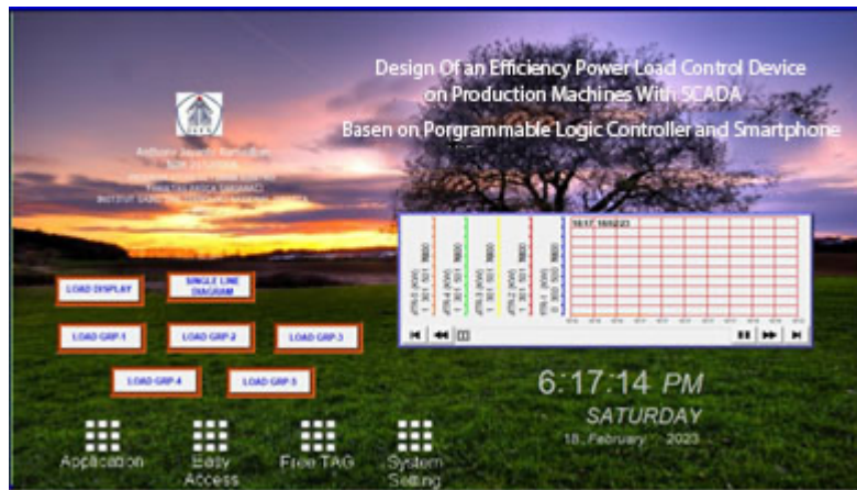
Figure 12. HMI display when connected to PLC
