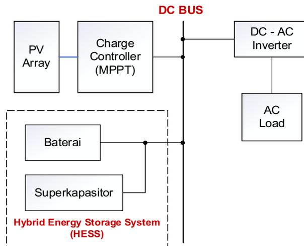
**Picture 2. Photovoltaic Battery Storage with Supercapacitor Schematic Diagram**
