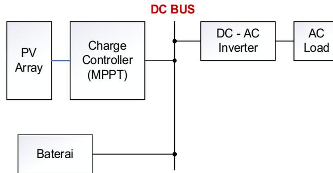
**Picture 1. Photovoltaic Battery Storage Schematic Diagram**
