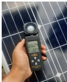
**Picture 5. Testing The Intensity of The Sunlight**
