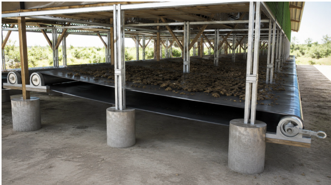
Figure 4. Manure Collection System Using a Tarpaulin in the House Design
