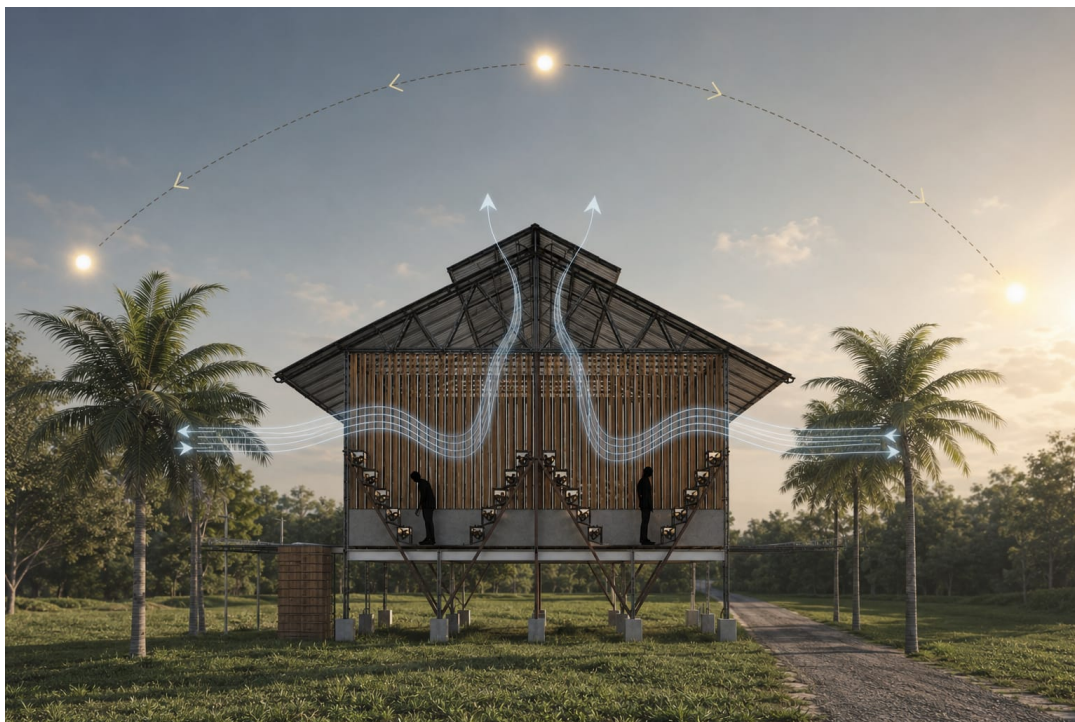
Figure 3. House Section and Direction of Air Movement
