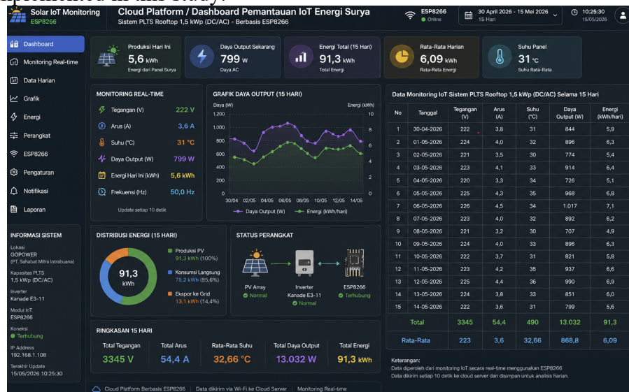
Figure 3. Solar Energy IoT Monitoring Cloud Platform / Dashboard
