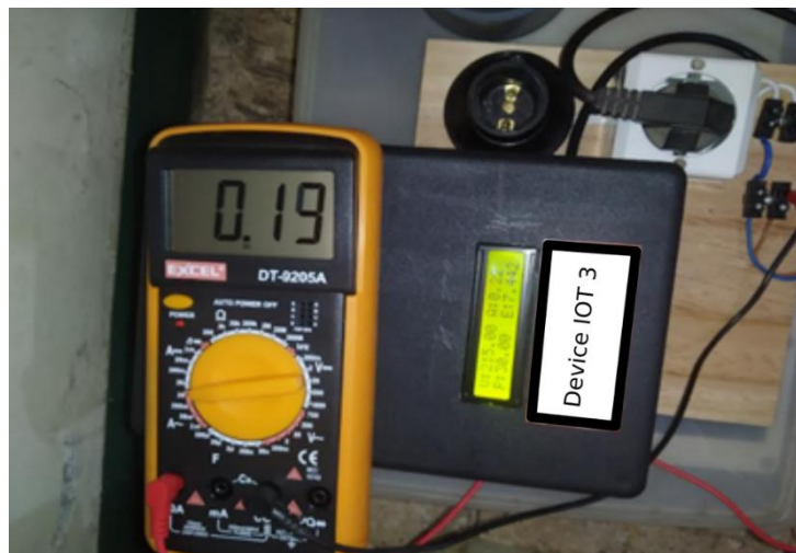
Figure 2. Manual Measurement of Electrical Current Using an AVO Meter
